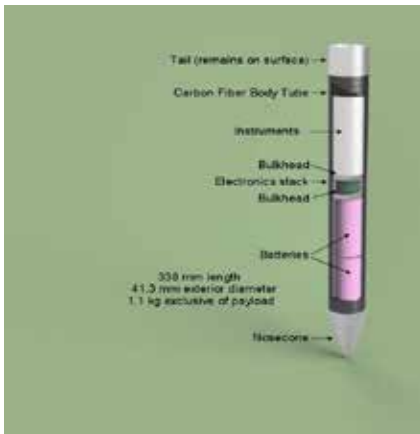
Figure 1: Cutaway drawing of a 388-mm long Mote penetrator designed to penetrate 1 to 2 meters into the lunar regolith.
