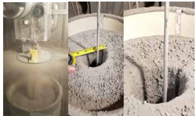
Figure 2: LISTER pneumatic drilling of lunar regolith analog BP-1 in a vacuum chamber and the regolith is directed out radially using a Dust Deflector (left). The top of the bore hole measures ~80-100 mm in diameter for a rocky regolith mixture (middle and right).
